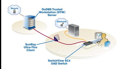
In this diagram, the SwitchView SC4 UAD switch supports the DoDIIS Trusted Workstation and the secondary unsecure workstation with a DVI-I interface, USB keyboard and mouse, and audio peripherals.
